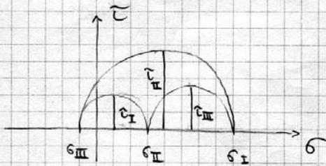
$$\max \left\{ \frac{|\sigma_I - \sigma_{II}|}{2}, \frac{|\sigma_{II} - \sigma_{III}|}{2}, \frac{|\sigma_I - \sigma_{III}|}{2} \right\} = \tau_{max}$$
