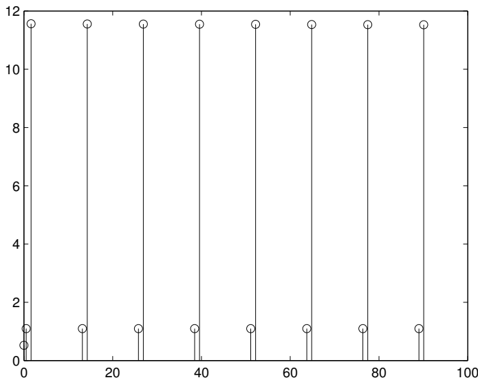
Figure 1. Self triggered control with \vartheta_1 = 0.99 and \vartheta_2 = 0.009 : (a) x_1 ; (b) x_2 vs time
