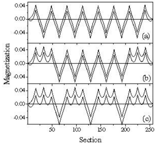
FIG. 4: Simulated magnetization of a  $N = 255$  Josephson junction 15  $\pi$ -loop array with  $\beta_L = 0.04$  and  $\alpha = 0.25$ : (a) solution with one unpaired paramagnetic half flux quantum, top curve  $\eta = 0$  bottom curve  $\eta = 0.1$ ; (b) solution with 10 paramagnetic half flux quanta, top curve  $\eta = 0$  bottom curve  $\eta = 0.5$ ; (c) solution with 12 paramagnetic half flux quanta, top curve  $\eta = 0$  bottom curve  $\eta = 0.7$ .
