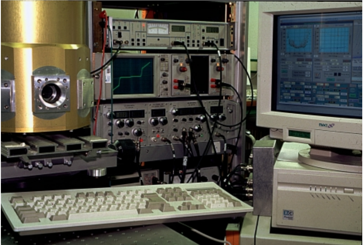
Figure 4. Photo of the experimental set-up controlled with IRTECON system: quasi-optical cryostat at the left, bias supply unit in the center (at the background) and data display at the right.
