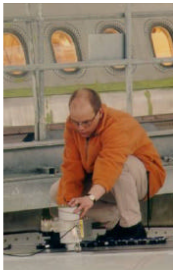
Figure 3. Aircraft fuselage testing using a mobile SQUID system with a x-y-scanner. The flexible scanner is affixed to the fuselage with suction cups. The SQUID is scanned in a meander-like path, thus yielding an eddy-current map of the fuselage section under test.
