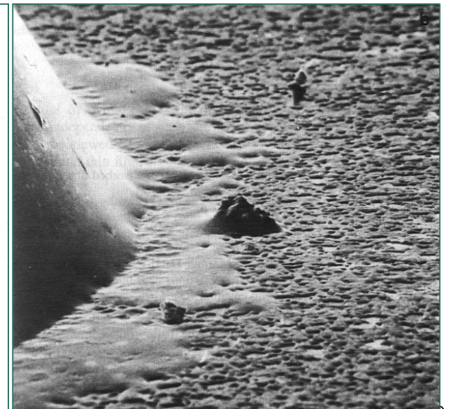
SEM picture of a drop of cooled glass on Fernico metal. \times 130
