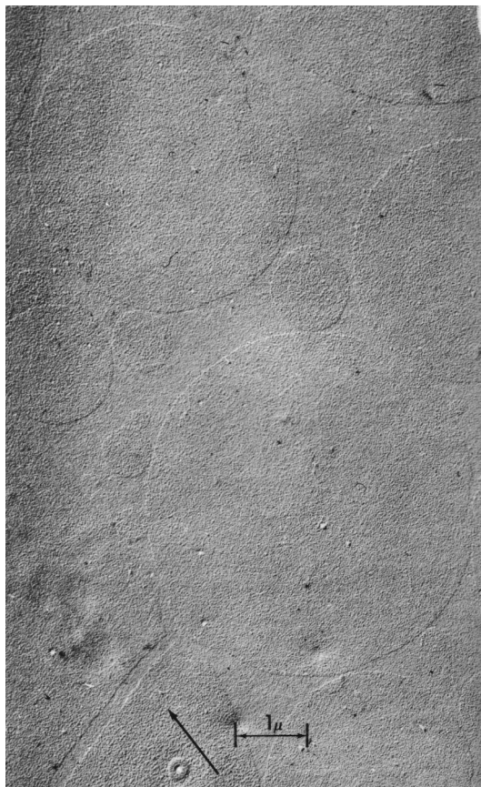
Fig. 3-46: Circular islands of condensed phase, one monolayer thick, in a sea of the uncondensed monolayer phase. Electron micrograph of a Langmuir-Blodgett monolayer of stearic acid at 10 mN/m, originally spread on water. From [Ries, H. E., Jr., and Kimball, W. A., Nature , 181 , 901 (1958).]
