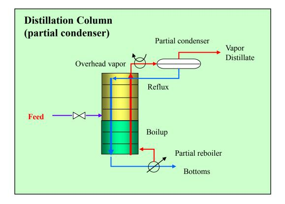
If the liquid reflux is obtained from a partial condenser, then the reflux is produced as the liquid in equilibrium with the vapor distillate in the condenser.
