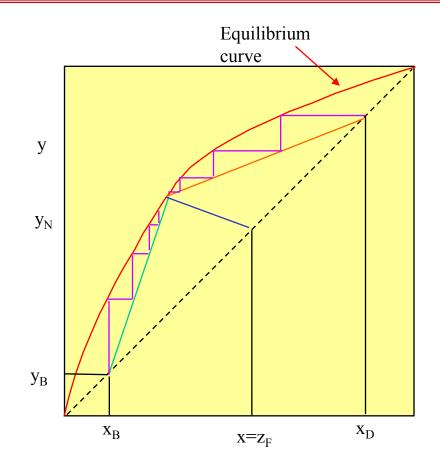
By returning no exiting vapor as reflux and no exiting liquid as boilup the operating line intersection is as far to the left as equilibrium allows. Although this is the minimum amount of reflux, it takes infinite stages (note the pinch point between the operating lines and equilibrium).
