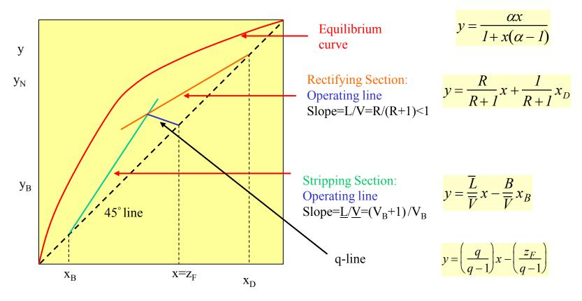
To carry out the algebraic method we need to determine the slopes of the operating lines algebraically. This can be done finding the intersections between the q-line and equilibrium curve, and the q-line and the rectifying section operating line.
