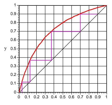
Minimum number of stages is determined by stepping off between the equilibrium curve and the 45 degree line. The result is 3.2 stages.
