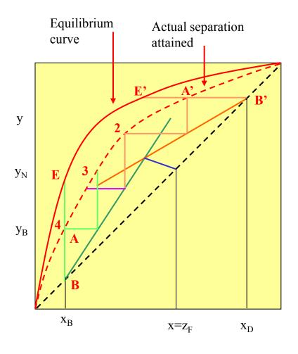
Component distribution obtained less than theoretical limit described by equilibrium The Murphree Plate Efficiency gives the ratio of the actual composition difference between two sequential plates, and that predicted by equilibrium.
