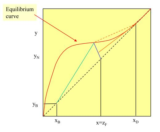
Although this is the minimum amount of reflux, it takes infinite stages (note the pinch point between the operating lines and equilibrium).
