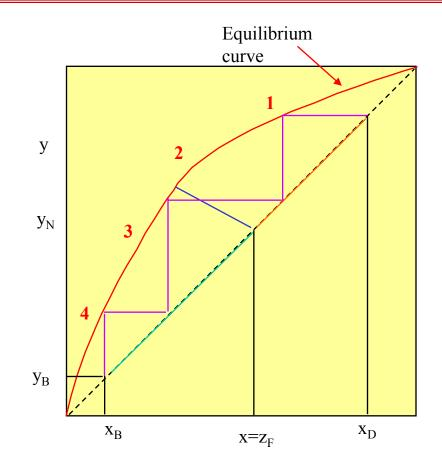
By returning all the exiting vapor as reflux and all the exiting liquid as boilup the operating lines have slope of one. Although this is the minimum number of stages, no product is produced (note the feed must then go to zero).
