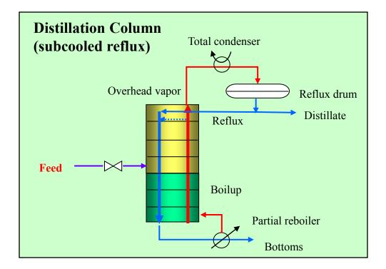
If the liquid reflux is colder than the bubble-point temperature, then it will condense some vapor in the top stage. This changes the reflux ratio to the internal reflux ratio.
