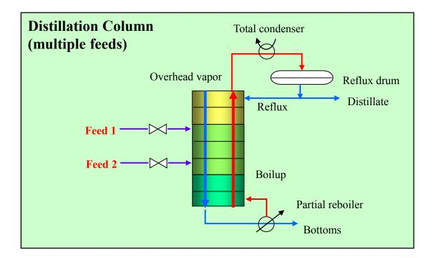
The McCabe-Thiele method for cascades can be applied to systems with more than two sections. Here, we show a cascade with 2 feeds: A 3 section cascade.
