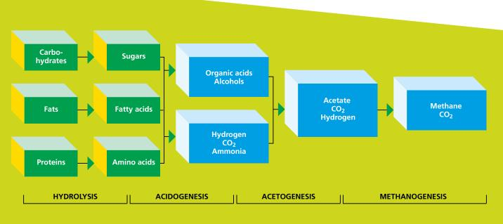
Fig. 11. Steps in anaerobic digestion.
