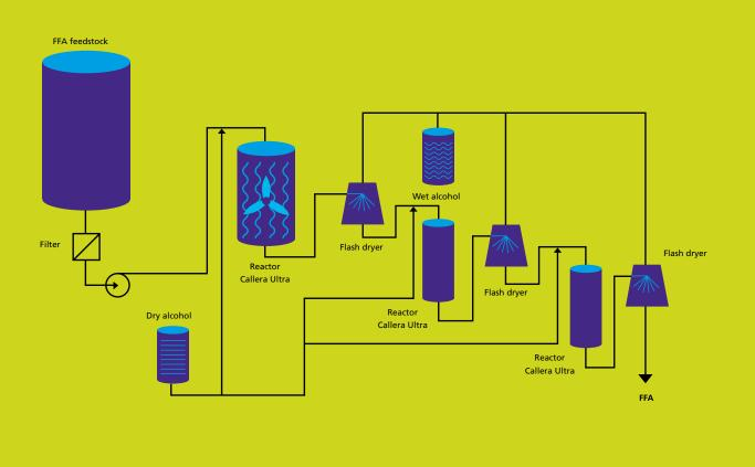
Fig. 10. Continuous biodiesel production from FFA using packed-bed reactors loaded with the immobilized lipase Callera™ Ultra IM produced by Novozymes.
