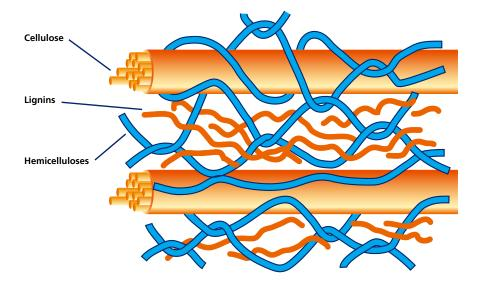
Fig. 6. Substrate complexity of lignocellulose.
