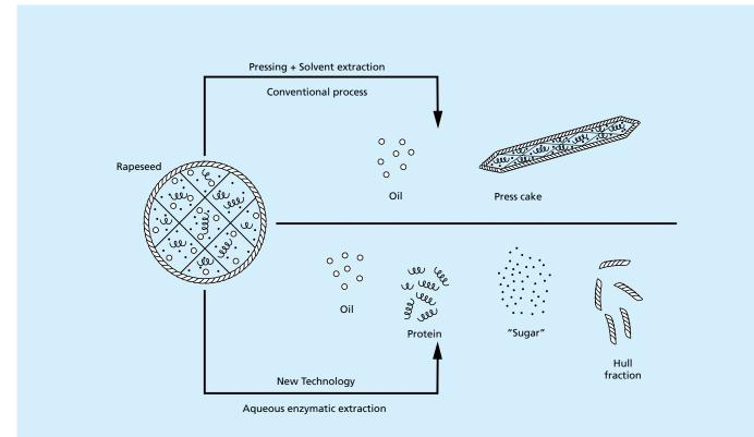
Fig. 12. Conventional process versus aqueous enzymatic extraction.
