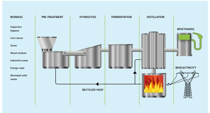
Fig. 8. General process flow for second-generation ethanol production.
