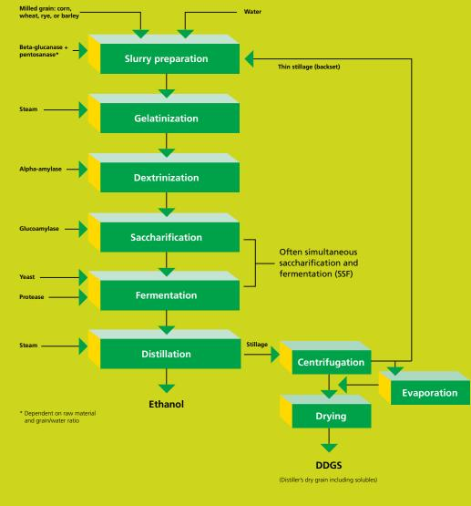
Fig. 4. Main process stages in dry-milling alcohol production.
