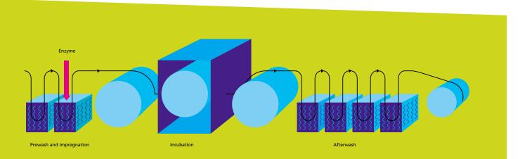
Fig. 2. A pad roll process.
