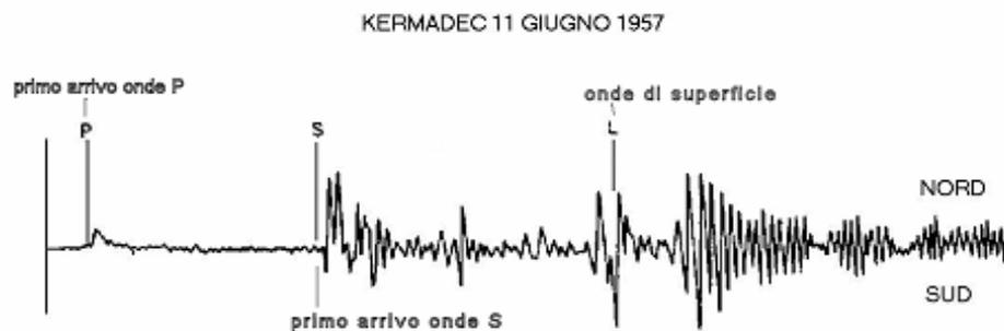
**Figura 2.** Tipico sismogramma registrato in superficie a grande distanza. (*typical seismogram recorded at long distance from epicenter*)
