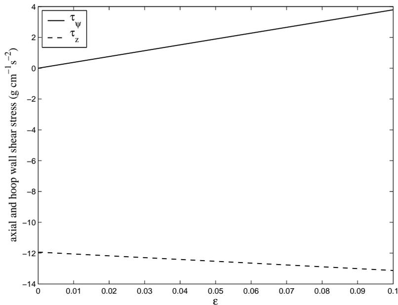
Figure 4. Amplitude at  $t = 0, z = 0$  of the axial ( $\tilde{\tau}_z$ ) and hoop ( $\tilde{\tau}_\psi$ ) wall shear stresses as functions of  $\epsilon$ . The plots refer to the maximum values with respect to  $\psi$ .
