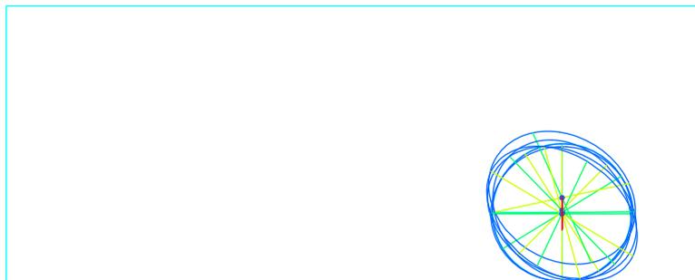
Figure 6: Without friction the body oscillates but does not move forward while the center moves on a vertical line.
