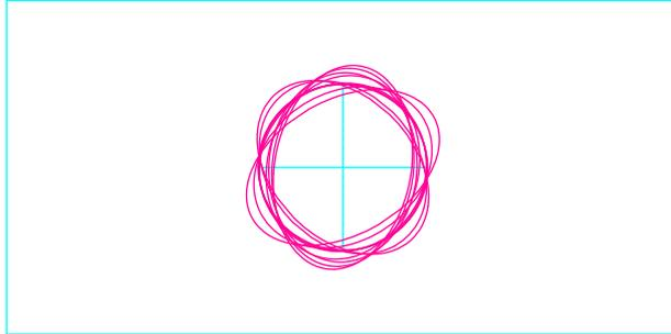
Figure 7: Evolution of the relaxed shape generated by an oscillating contraction with rotating principal axes.
