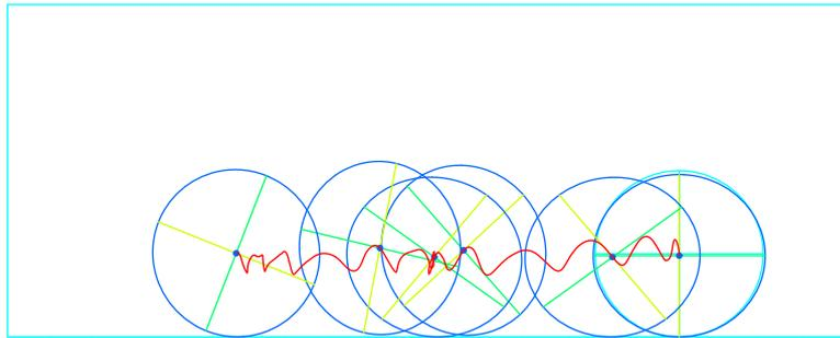
Figure 5: Trajectory of the center and some frames in a motion from right to left, driven by an oscillating contraction with rotating principal axes.
