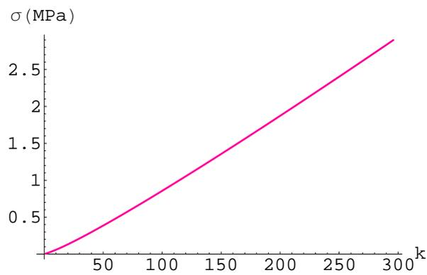
Figure 3.9: Cauchy stress versus relaxed radius to thickness ratio (inner pressure  $p = 10$  kPa)
