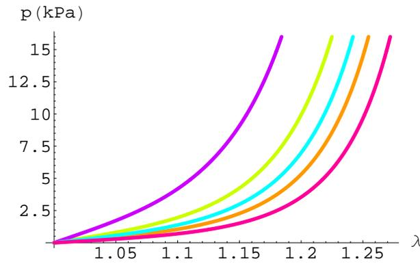
Figure 3.8: Inner pressure versus hoop stretch ( $k = 50, 107, 152, 200, 300$ , from left to right)
