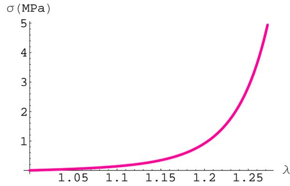
Figure 3.7: Cauchy stress response given by Fung strain energy
