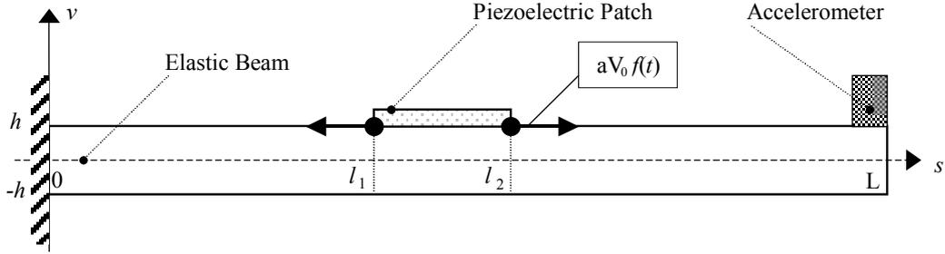
Figure 1: Schetch of the cantilever equipped by piezo-patch and accelerometer
