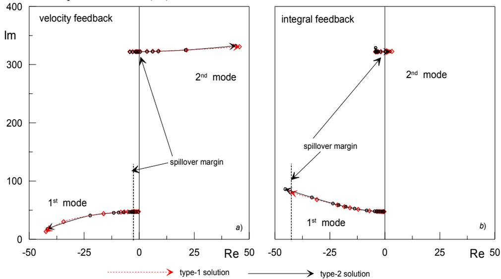
**Figure 2:** Root-locus of 1<sup>st</sup> and 2<sup>nd</sup> mode: a) velocity output-feedback b) integral output-feedback
